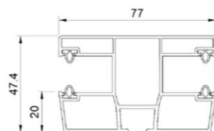
Divisive (PVC) roller guide - RS revision from the inside. MK939
